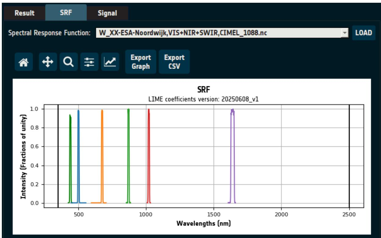
Figure 14: SRF tab showing CIMEL SRF.
