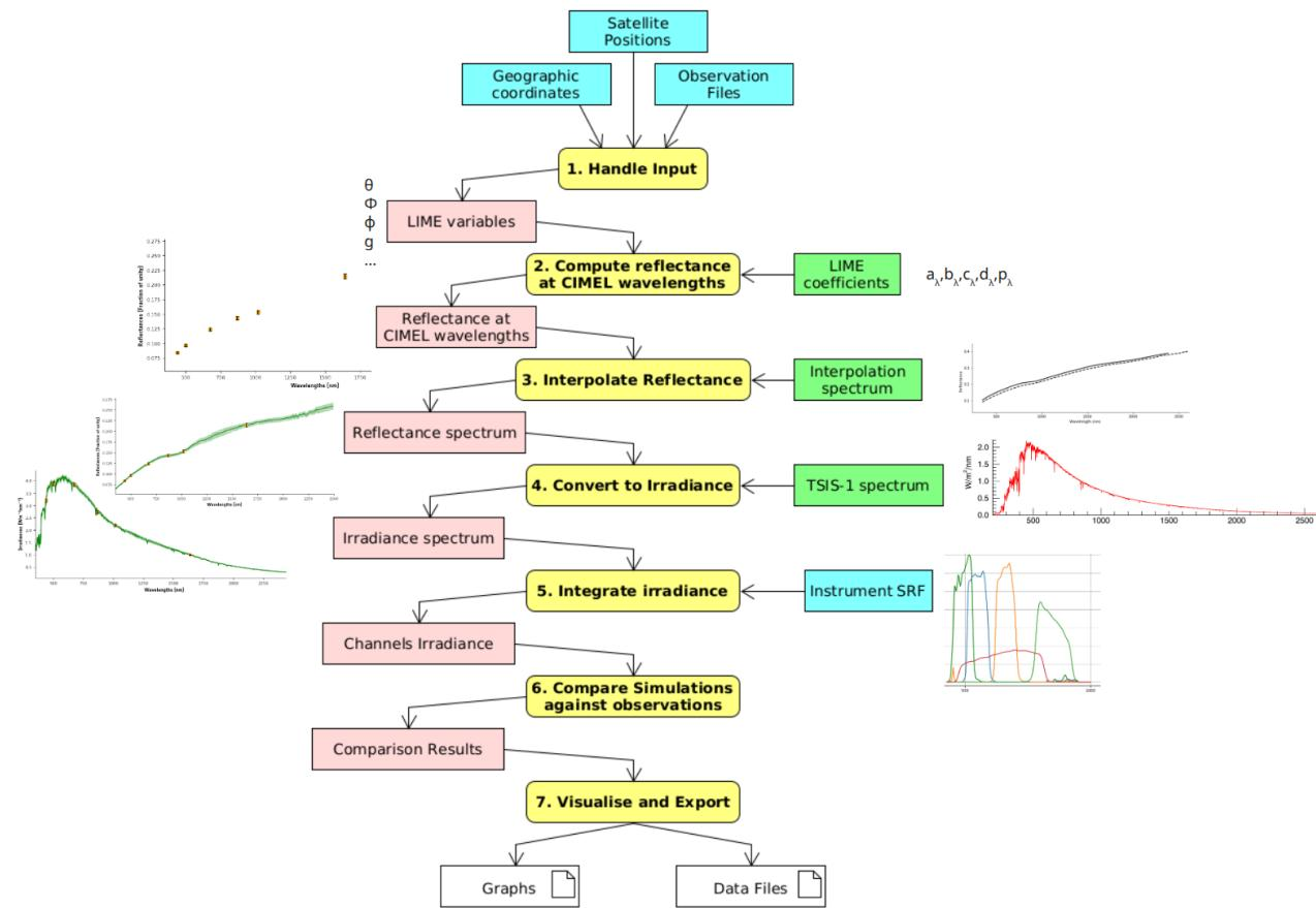
*Figure 1: Activity diagram of the Simulation & Comparison Workflow.*
